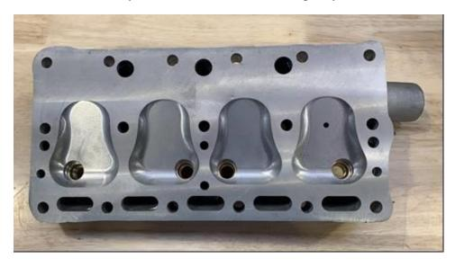
They will also fit other BSA's with the 9hp and should fit 10hp 4 cylinder engines.
