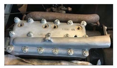
All machining is by CNC and this includes the combustion chambers/valve/spark plug area. This has ensured that all four combustion chambers are 100% identical and as per the factory drawing (unlike originals). Originally the combustion chambers were cast (no CNC back in the 1930's).
